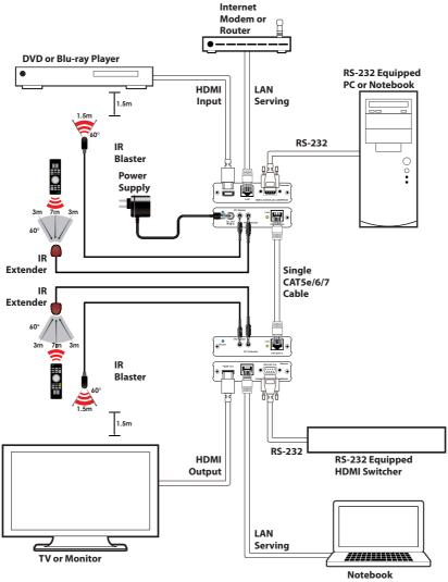
Note: Only the Transmitter unit needs to be powered and can power the Receiver unit via PoC.
