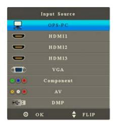
When it is **Off**, the OPS computer will not be started when the interactive panel is started. (Press **Source** and the list of signal sources does not show **OPS-PC**.)
