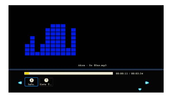
➤ Press **DISPLAY** to show the operation function menu. Press **I** to select a function and press **OK** to use the function.
