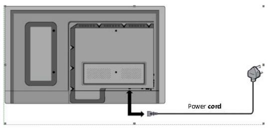
**Step 2** Turn on the rocker switch at the bottom of the interactive panel (next to the power port) to enable power supply. In this case, the indicator is in red.
